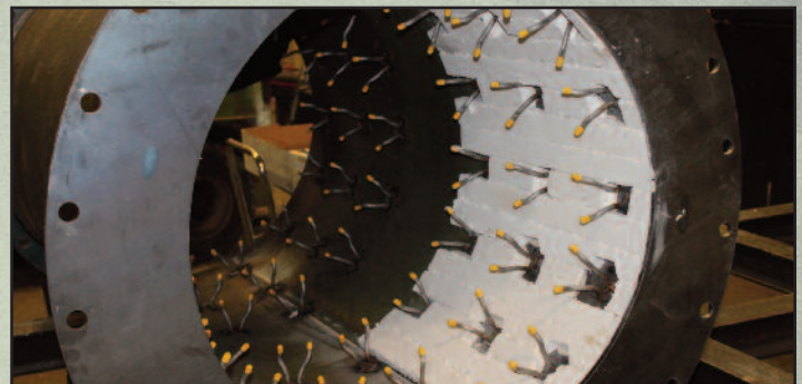
Fabricated pipes are being prepared for refractory.
