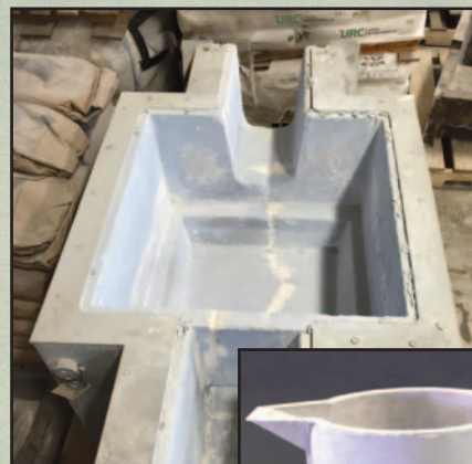
Used filter bowl to be relined with UNI-CAST FS-6A
