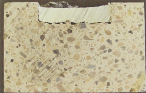
UNI-SHIELD 70A cup tests with various alloys show little to no penetration.
